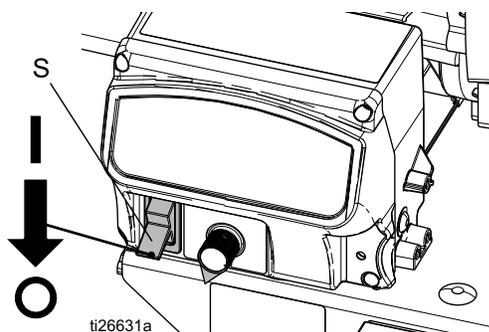
2. Ground sprayer (see **Grounding**, page 10). Plug the power cord into a dedicated 15 amp, 120 V circuit (or a 10 amp, 230 V circuit, depending on model).
