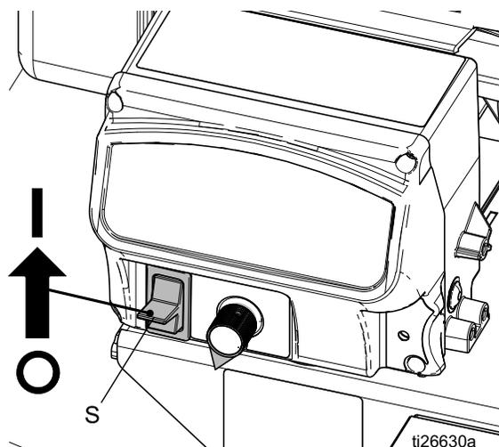
5. Turn flow adjustment knob (H) until desired flow is reached. Turn clockwise to increase flow, counterclockwise to decrease flow.
